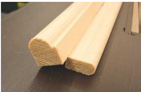
▲ Pic.26 Mould the parting and staff bead; cut and fit the parting beads with the outer sash
